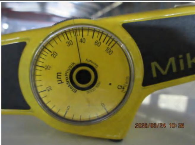
Pic.17 Coating thickness check
