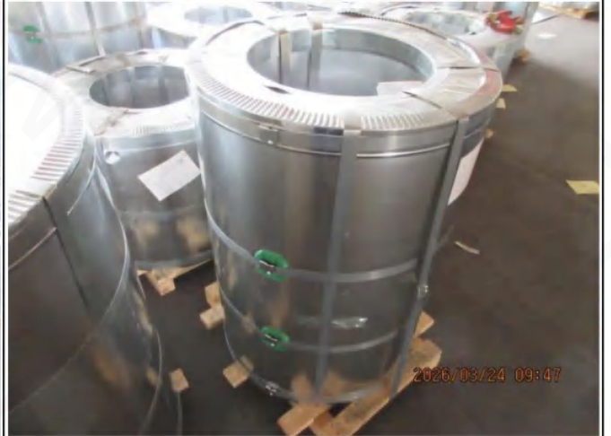
Pic.4 Marking and package check
