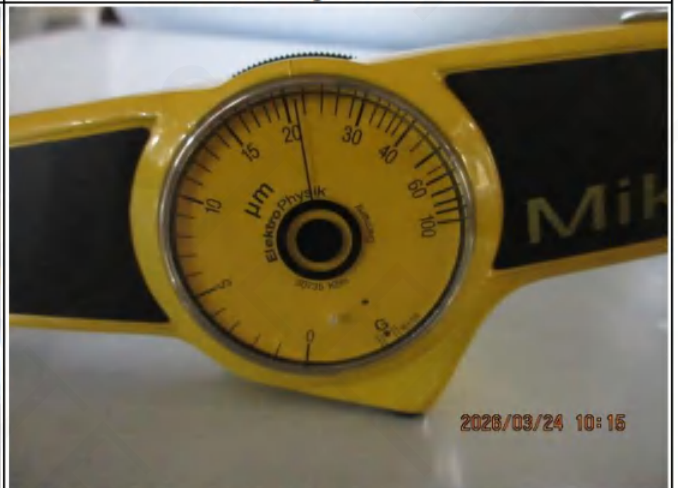
Pic.18 Coating thickness check
