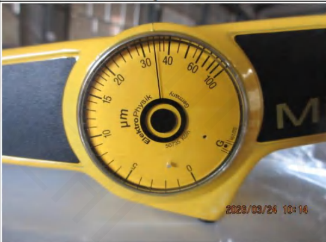
Pic.17 Coating thickness check
