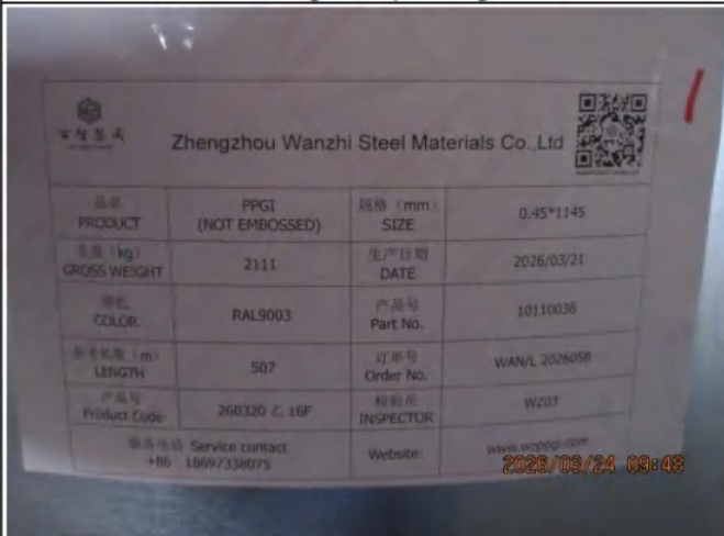
Pic.5 Marking and package check
